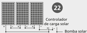
PANEL SOLAR: 3 x 340W
