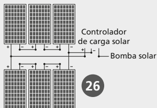
PANEL SOLAR: 6 x 340W
